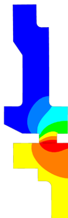
FEA Optimized seal face for stable dry running
