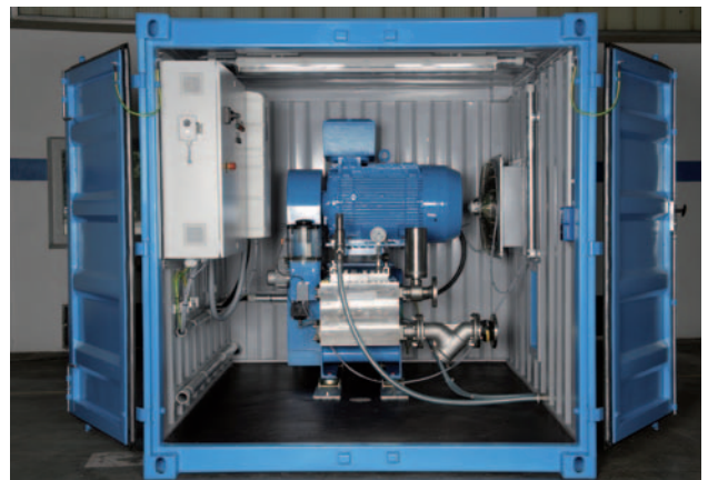
ABEL HPT as ready-to-use, mobile container pump
