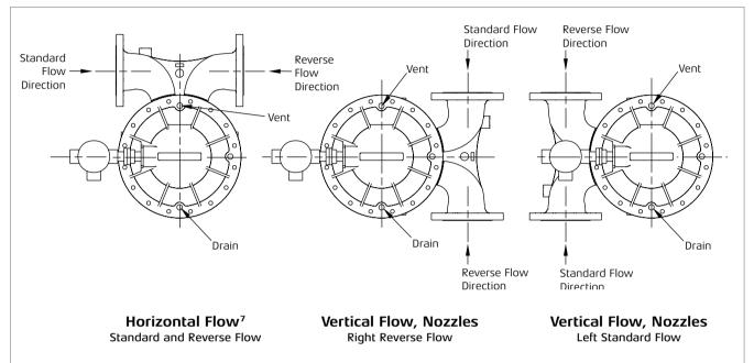
**Note:** Drain must always be in down position as shown. Vent source should always be the highest vertical point of the meter. The cover vent may not always be at this point and an alternate vent source should be used.
