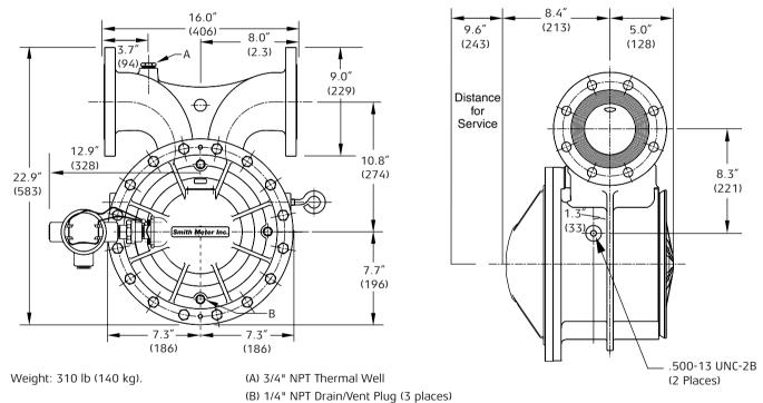
**Note:** Dimensions – Inches to the nearest tenth (millimeters to the nearest whole mm), each independently dimensioned from respective engineering drawings.
