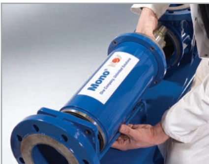
4. Lift rotor and stator out of the pump
