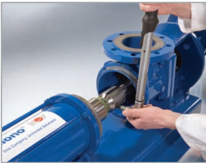
4. Lift rotor and stator out of the pump
