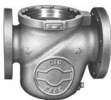
Viking Lid-Ease Simplex Strainers are designed with a weatherseal lid to protect the breech lock area from exterior elements and prevent air infiltration into the pump suction. Strainers are also equipped with a drain plug for complete draining of strainer if needed.
