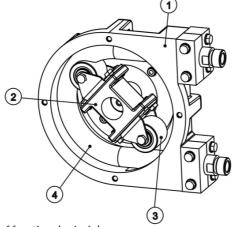
Fig. 1: Diagram of functional principle.1 Casing2 Rotor3 Rollers
