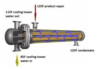
The temperature of the condensate can only fall below the vapor temperature of 120F (48°C) when all vapor in the condenser has changed into a liquid. That is termed subcooling and is the correct mode of operation for the condenser. IT IS IMPORTANT TO UNDERSTAND THIS.
