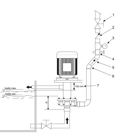
manually verify that all rotating parts are free to turn without abnormal friction by turning the motor cooling fan make sure that the power supply is compatible with the data shown on the pump motor identification plate connect the motor to the power supply via a magnetic/thermal control switch
