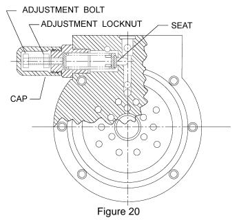
All PULSAR pumps incorporate a Hydraulic Bypass Valve which is an adjustable spring-loaded valve ported into the hydraulic cavity of the pump head. The valve is designed to protect the pump against excessive hydraulic pressure and will not limit or regulate system pressure. The valve is factory-adjusted for pressure as originally specified, or at 10% above the rated pump pressure.
