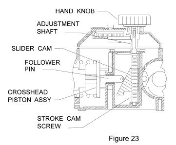
The hand knob linkage employs a slip type coupling which can be reassembled in either of two rotational orientations 180° apart from one another: therefore, the original orientation must be retained for reassembly so that pump calibration is retained.
