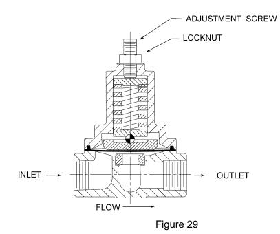
The Pulsafeeder diaphragm backpressure valve creates constant backpressure. A TFE diaphragm, offering maximum chemical protection and service life, seals spring and bonnet from product. This diaphragm seals directly on a replaceable seat.
