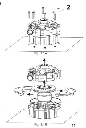
As described on paragraph no. 2 "Disassembling sequence", unscrew the connections (POS.1) and remove the HYDRAULIC PARTS from the MOTOR
