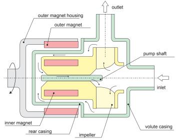
outer magnet to rotate together with its housing, the inner magnet assembly is dragged at the same speed. As a result the impeller, which is integral to it, is maintained in rotation.
