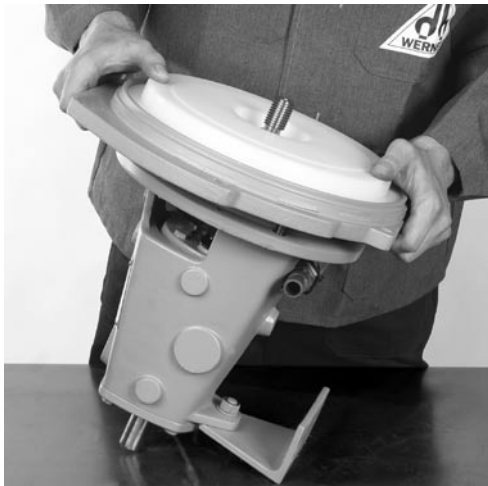
Fig. 7.53 Carefully slide the pre-assembled adapter over the bellows into the bearing housing centre and screw tight.
