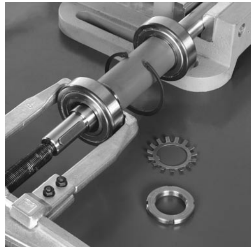
Fig. 7.31 Remove radial ball bearings by means of a removal device. The removed shaft nut and circlip are lying beside it.
