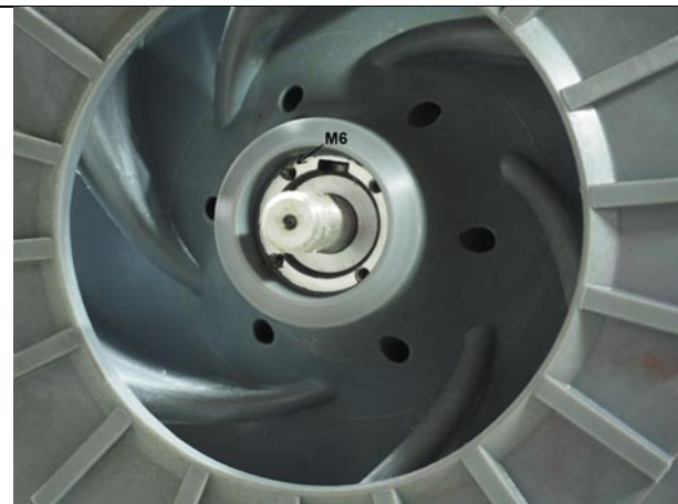
Fig. 4.17 Impeller with 4 threaded holes M6 in impeller bush.
