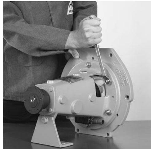
Fig. 7.13 Remove existing rinsing connections. Loosen hexagon nuts to separate bearing housing from the adapter.
