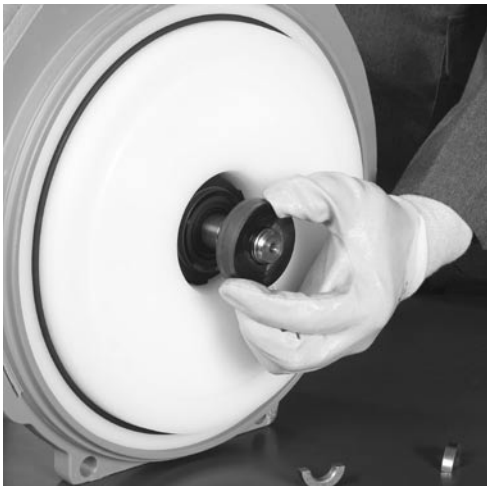
Fig. 7.12 Remove the multiple ring from the shaft using special tool (part 052) and remove the rotating seal ring.
