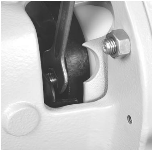
Fig. 7.61 Empty pump. If the pump is to go into storage, loosen hexagon nuts on the bellows. By loosening the nuts the bellows is keeping its elasticity.
