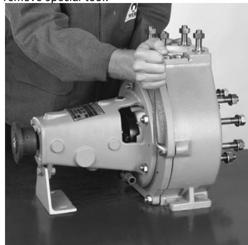
Fig. 7.58 Insert back pull-out unit into pump casing and screw it to annular casing using locking screws and hexagon nuts. For NEPE 100-65-315 and 80-50-315 the following applies: Centering is carried out via two drill sleeves (part 540).
