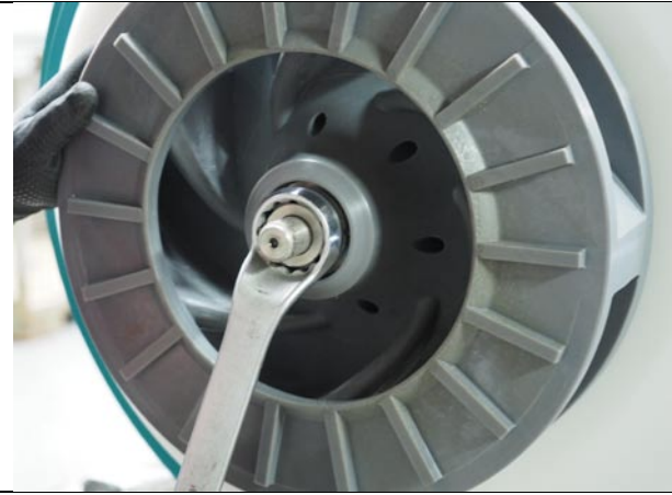
Fig. 4.15 ➤ Unscrew the hexagon nut (part 920.59) to the left.
