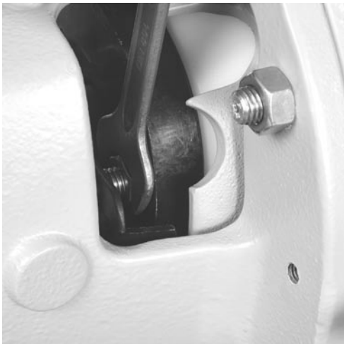
Fig. 7.59 Tighten hexagon nuts on bellows seat following instructions (⇒ section 6.1.4). Avoid excessive tightening!
