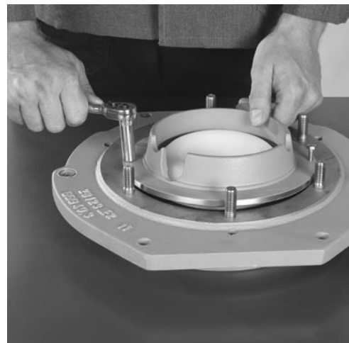
Fig. 7.17 Press the centering ring from the adapter using ejector screws and remove centering ring.
