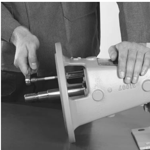
Fig. 7.26 Take shaft seal ring off the shaft. Remove the hexagon head bolts from the bearing cover. Remove bearing cover.
