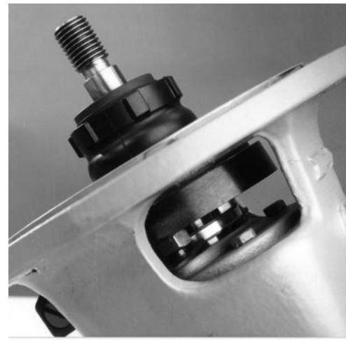
Fig. 7.50 Place pre-assembled bellows seat onto the grub screws.
