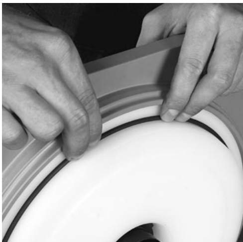
Fig. 7.55 Place casing seal (O-ring) onto the seal insert, make sure it is correctly positioned.
