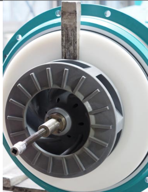
Fig. 4.18 If the impeller bush is stuck on the shaft journal due to corrosion, for example, please use the pulling device. ➤ Fix the pulling device to the impeller bush by using 4 hexagon head screws (M6). ➤ Remove the impeller by screwing in the spindle.
