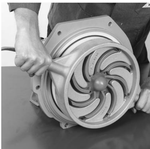
Fig. 7.57 Screw semi-open impeller with inserted O-ring onto shaft and tighten with special tool (part 051). Fix shaft beforehand.
