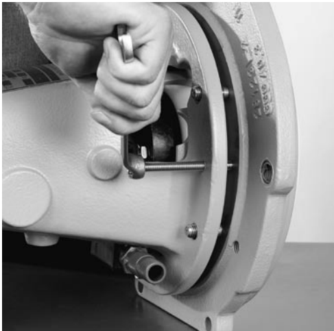
Fig. 7.14 Separate bearing housing and adapter using ejector screws. Pull out bearing housing with the shaft.
