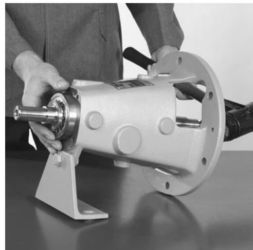
Fig. 7.27 Push shaft with radial ball bearings off the bearing housing by carefully beating against the front face of the threaded journal with a plastic hammer.
