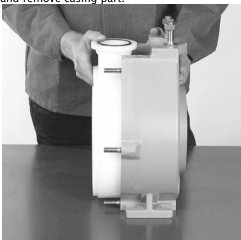
Fig. 7.34 Remove pump casing from annular casing.
