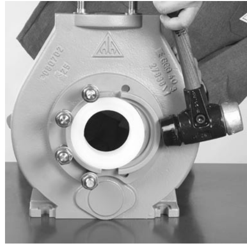
Fig. 7.36 Insert retaining rings on suction nozzle, then tighten studs.
