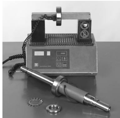
Fig. 7.38 Slide circlip over the shaft's waist, heat radial ball bearings and pull them onto shaft. In case of grease lubrication sealing discs must point inwards. Lubricate bearings according to operating instructions.
