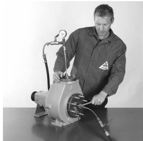
Fig. 7.60 Close pump nozzles tightly. Perform leakage test.
