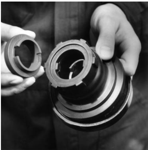
Fig. 7.49 Assemble bellows with stationary seal ring and bellows seat. Take care to line up grooves and cams on all three components.
