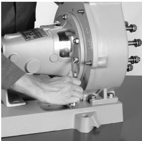
Fig. 7.8 Take away hexagon head bolts on bearing housing. Take away caps.
