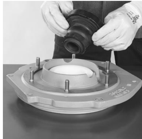
Fig. 7.15 Take bellows with stationary seal ring and bellows seat off the seal insert.
