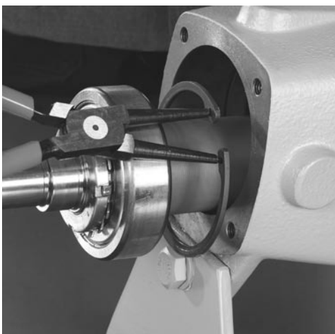
Fig. 7.28 When the bearing on the side of the motor lies exposed press the circlip together with a round nose pliers and remove it from the nut.
