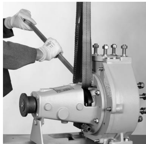
Fig. 7.9 Push off back-pull-out-unit from annular casing. Depending on liquid pumped take safety measures. Protect eyes! Danger of cauterization!
