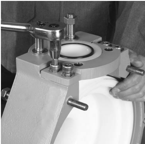
Fig. 7.37 Insert O-rings into nuts on suction and discharge nozzle. Slide casing part under the discharge nozzle and fix it. Attach all studs.
