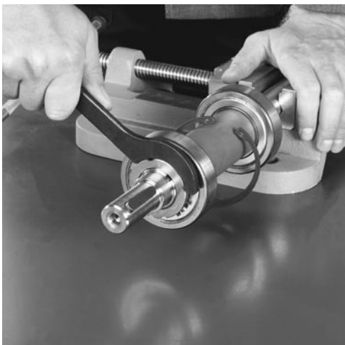
Fig. 7.39 Slide lockwasher onto shaft. Tighten shaft nut with spanner. Lock shaft nut with lockwasher.
