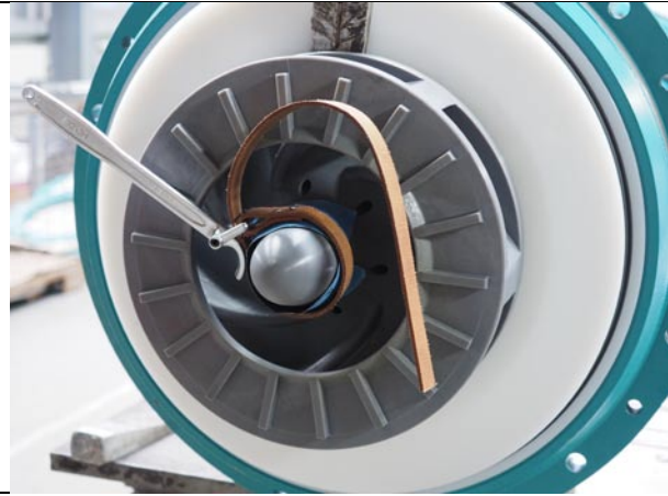
Fig. 4.14 ➤ Unscrew the impeller cap (part 260) to the left using a strap spanner and sandpaper for better adhesion. Insert the wedge behind the impeller.
