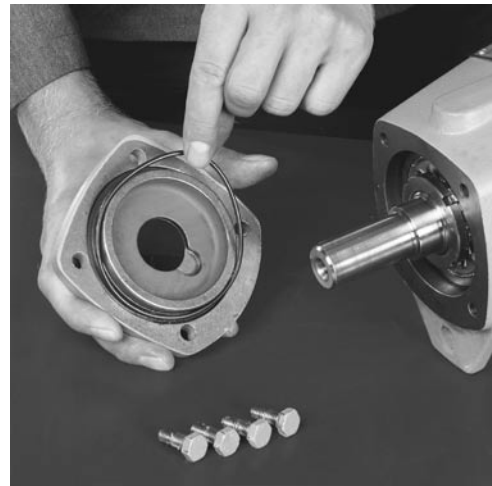
Fig. 7.25 Take off bearing end cover and O-ring.
