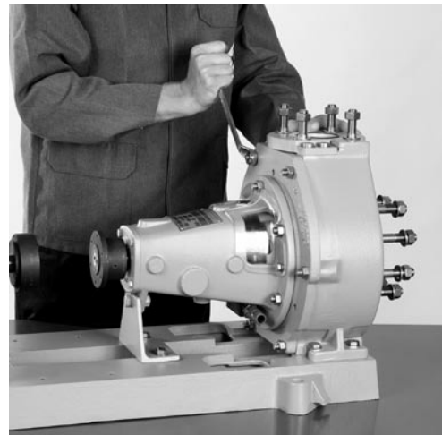
Fig. 7.7 Take away hexagon nuts on adapter / annular casing and hexagon head bolts on support foot.
