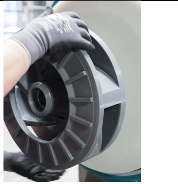
Fig. 4.19 Normally the impeller can be pulled off the shaft end by hand.
