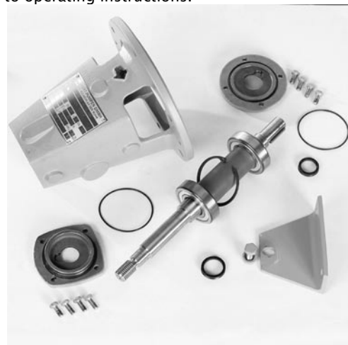
Fig. 7.40 Bearing housing, pump shaft with radial ball bearings and circlip, bearing covers with O-rings and shaft seal rings.
