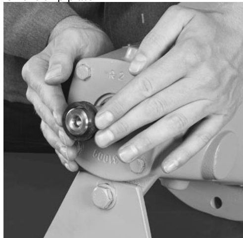
Fig. 7.23 Remove key. Take shaft seal ring off the shaft.
