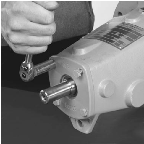
Fig. 7.24 Remove screws at bearing end cover.
