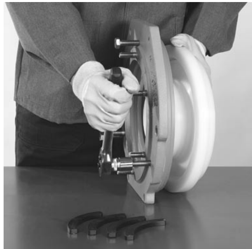
Fig. 7.19 Separate adapter and seal insert using ejector screws.
