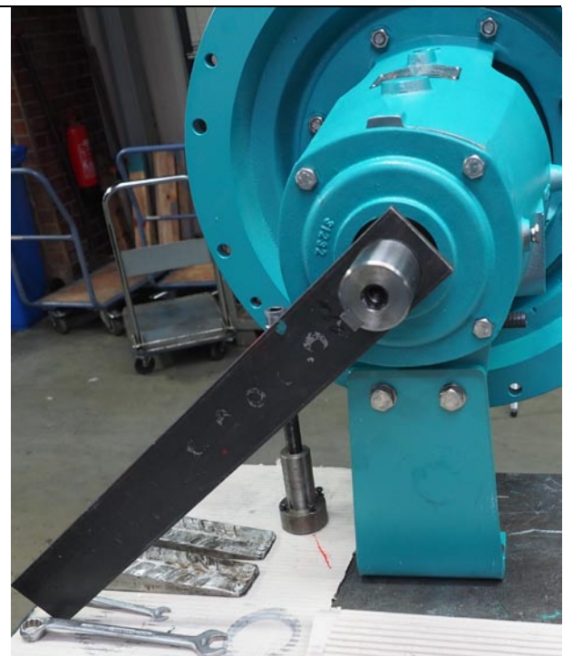
Fig. 4.13 ➤ Fix the shaft to the shaft journal or coupling to prevent twisting (tool 6).
