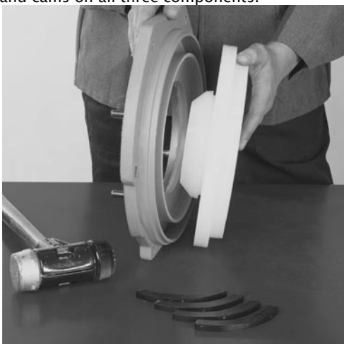
Fig. 7.51 Insert seal ring into adapter and secure it with the retaining ring made up in four-parts.
