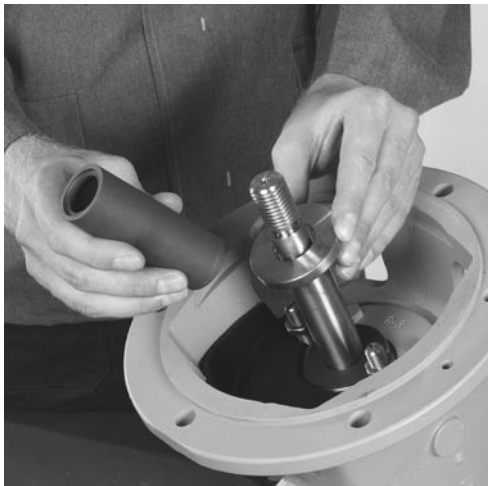
Fig. 7.20 Pull shaft wearing sleeve with O-ring and locking disc system from the shaft.
