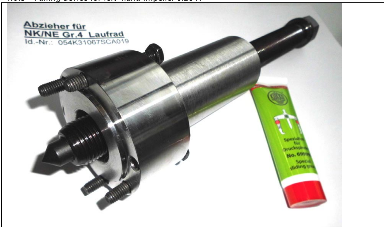
Fig. 4.10 Pulling device, WERNERT identification number: 054K31067SCA019
