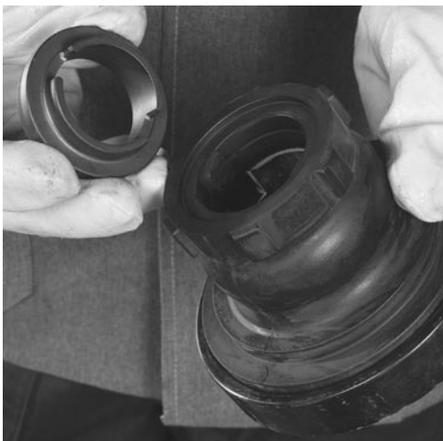
Fig. 7.16 Loosen connection of stationary seal ring, bellows and bellows seat by means of easy pulling.
