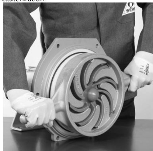
Fig. 7.11 Loosen the semi-open impeller in sense of rotation of the pump using special tool (part 051). Fix shaft beforehand. Disassembly left-hand impeller size IV ⇒ section 4.6.3.
