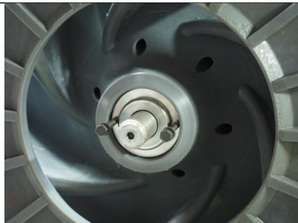
Fig. 4.16 ➤ Screw 2 M6 hexagon head screws into disc (part 550.1) and remove the disc.
