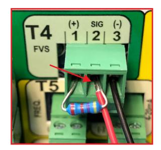
**Step 3.** Trim the bare and connect the RED WIRE to the left positive PIN 1 and the BLACK WIRE to the right negative PIN 2 on the FREQUENCY terminal on the MS-6 circuit board.
