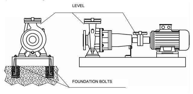
Long-coupled pumps have been pre-aligned with the motor prior to shipment. If pump units receive rough treatment during shipment, they can become misaligned. The flexible coupling is not designed to compensate for misalignment. Improper alignment will cause vibration and premature bearing failure.
