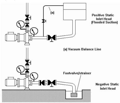
If the supply vessel is under vacuum, a pressure balancing line should connect the supply vessel and the pump inlet port.
