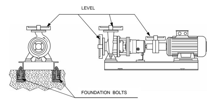
Close-coupled pumps have been aligned prior to shipment and if they turn freely by hand, no further adjustments are necessary.
