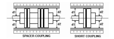
**IMPORTANT NOTE:** The straight edge method checks static coupling alignment, not shaft alignment. It relies for its accuracy on the accurate alignment of each coupling half on its shaft. The straight edge method is a useful preliminary check, but should not be seen as an effective final alignment method.
