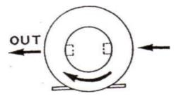
**IMPORTANT:**do not run the pump in reverse. Reverse rotation will lead to accelerated wear and eventual failure.
