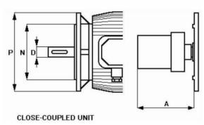
Insert key into shaft keyway and locate the outer magnet on the shaft in accordance with dimension A shown above, and tighten the grub-screw. Fill the bearing housing with oil to the middle of the sight glass.
