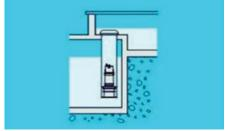
If the water level on the outlet side of the pump varies considerably flap valves can be installed.
