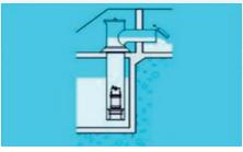
If the water level on the outlet side of the pump varies considerably flap valves can be installed.
