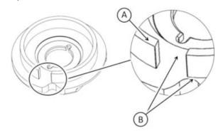
Do not retouch any other surface of the piston by any mean as it can degrade pump performance and reliability. In particular, do not round or attenuate disc wall edges.
