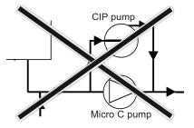
Indeed, in this case, the pressure at the inlet of the Micro C pump is lower than the pressure at the discharge and the piston remains forced against the cylinder. Therefore, the Micro C pump no longer provides a passage. Its efficient cleaning can no longer be ensured and the cylinder/piston pair will become prematurely worn.
