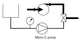
The Micro C pump is stopped when cleaning the installation.
