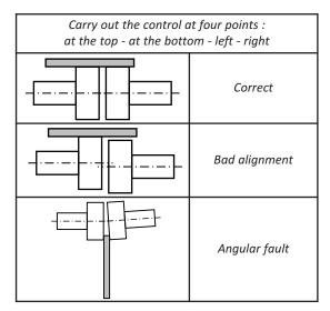
Controlling the alignment at each stage of the installation is important to be sure that none of these stages have generated stresses on the unit or the pump :
