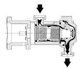
• A centrifuge pump is used for CIP cycles. This centrifugal pump is placed upstream of the Micro C pump.
