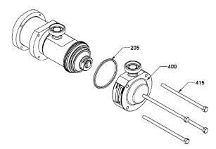
5.5 Trunk disassembly/reassembly
