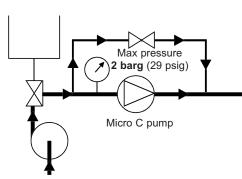
It is preferable not to run the Micro C pump during CIP although low speed (< 100 rpm) is acceptable by alternating start/stop operation.
