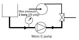
We recommend limiting the rotation speed of the Micro C pump.
