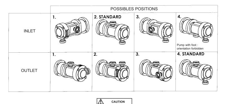
All other ports orientations are not totally drainable. When inlet port is in position 1, 3 or 4, take care to not clog the vent and to protect it from outside.
