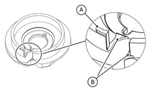
Before putting back the piston on the pump, eliminate these asperities by filing and finishing with fine sandpaper (No 320 grain or equivalent), taking care of not scratching any other surface around. Piston must then look as follows :
