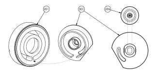
Place thread locking adhesive (Loctite® 243\* or equivalent) on the thread of the transmission hub 596.
