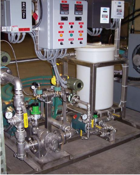
Utilizing ECO GA12 Flanged Pump to pump resin.
