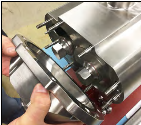
Figure 128 - Install pump cover
