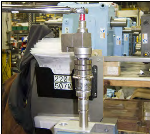
Figure 179 - Torque down locking nut
