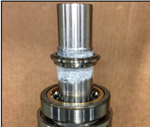
Figure 171 - Place race on shaft
