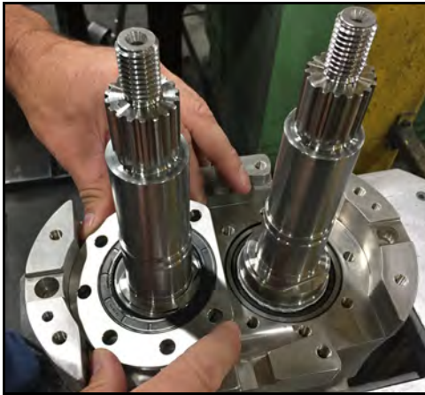
Figure 144 - Remove bearing retainer
