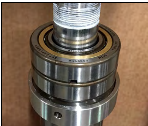
Figure 173 - Second bearing installed
