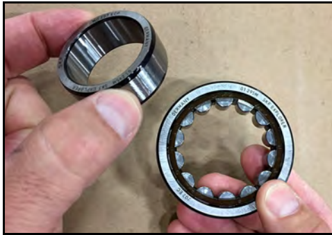
Figure 174 - Remove race from bearing
