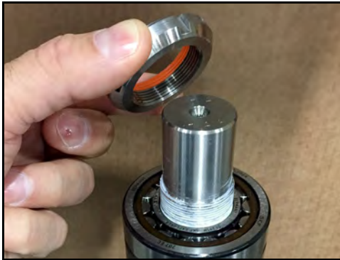
Figure 178 - Place locking nut onto shaft
