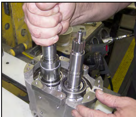
Figure 189 - Place drive shaft in bore
