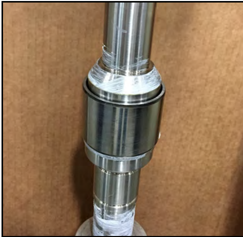
Figure 156 - Inner race installed on shaft
