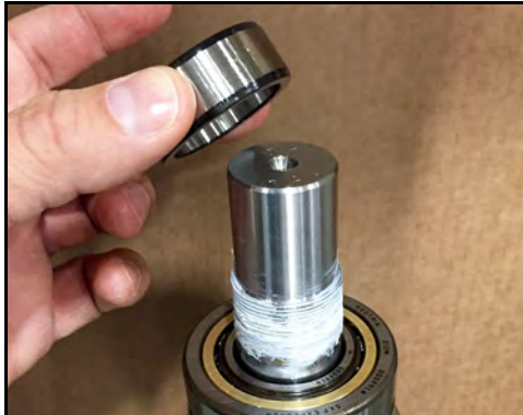
Figure 175 - Place race onto shaft
