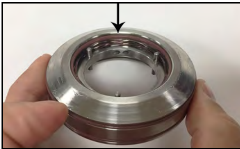
Figure 70 - Carrier-to-seal O-ring installed
