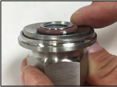
Figure 115 - Belleville washer installed
