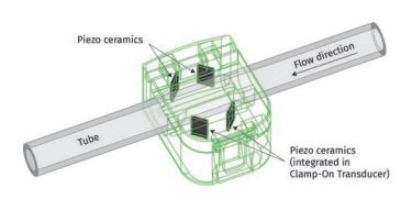
A typical transit time flow measurement system incorporates two piezo ceramics that act as both ultrasonic transmitter and receiver. The flow measurement is conducted by alternately transmitting and receiving an ultrasonic pulse between the two transducers and by measuring the transit time difference that it takes for the pulse to travel between them.
