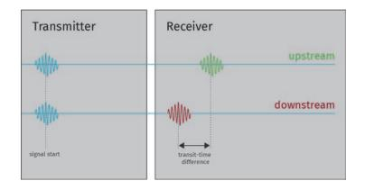
The picture on the left shows the transmitting impulses and the resulting received signals. The transit time difference is determined through the received signals.
