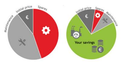
The shown comparison of cost over a period of 5 years on a DN100 pinch valve feeding abrasive slurry. The valve operates 4-6 times/hour. The conventional valve is a stainless ball valve with PTFE seats.
