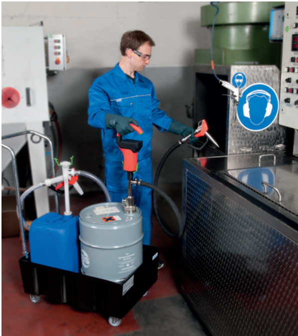
High mobility due to battery motor.
