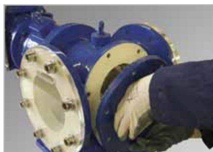
6. Inspect/replace cutters, spacers and shafts
