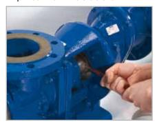
3. Unscrew and remove tie rods
