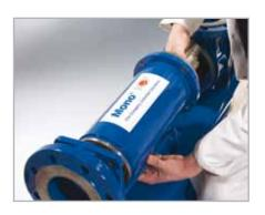
2. Remove new split coupling rod sleeve
