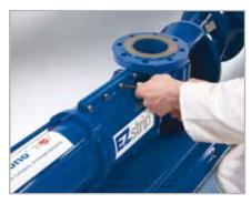
2. Remove rags from the coupling rod area and simply bolt back together
