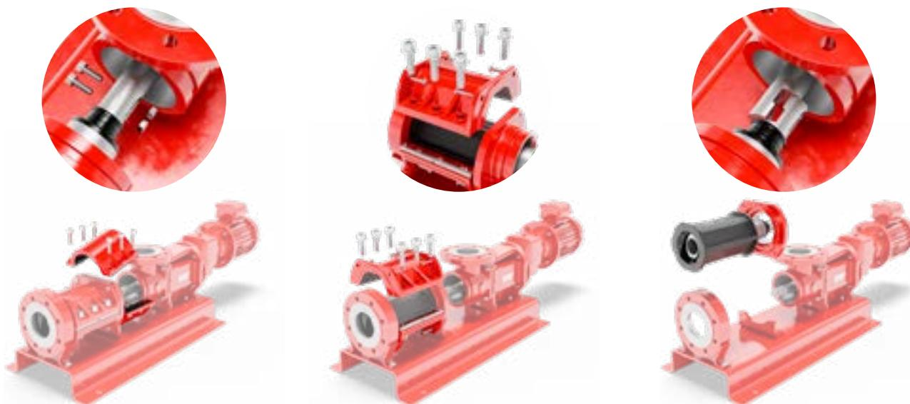
Open the service access and loosen the two bolts on the split drive shaft.
