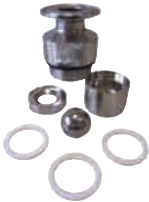
Clamp-connection and ball valve in SS316L with Ra 0.8, PTFE gaskets (FDA approved)
