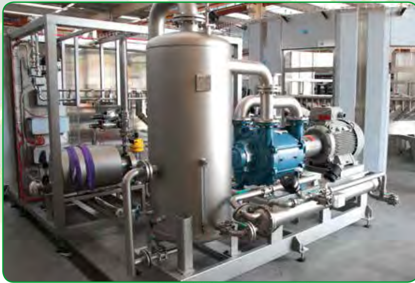
Bottling: vacuum pumps used to suck in air in the glass bottles filling systems.
