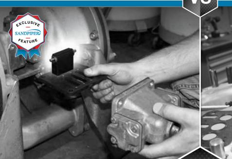
The Air Motor's Pilot Valve is the Most Often Serviced Part on an AODD Pump
