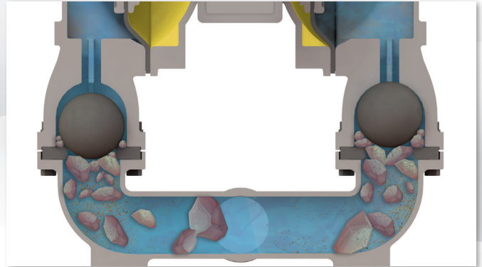
Large solids cannot pass through pump, affecting operation
