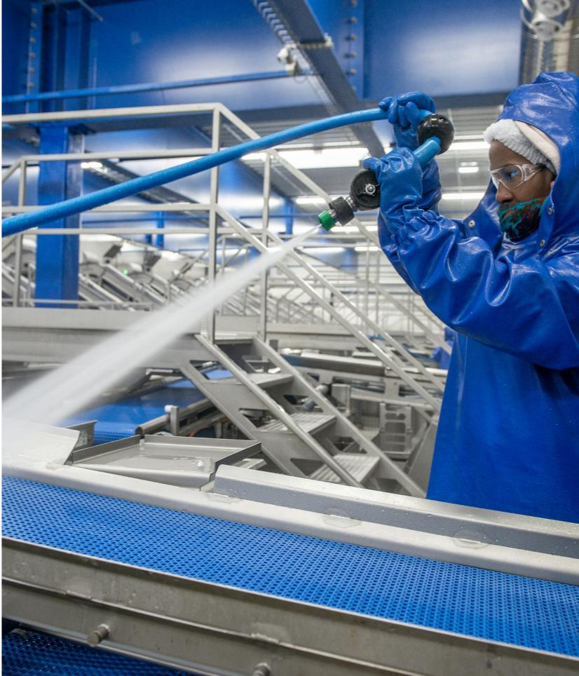
Low-pressure cleaning with boosted water safeguards the processing environment against microorganisms thereby eliminating the recontamination of surfaces
