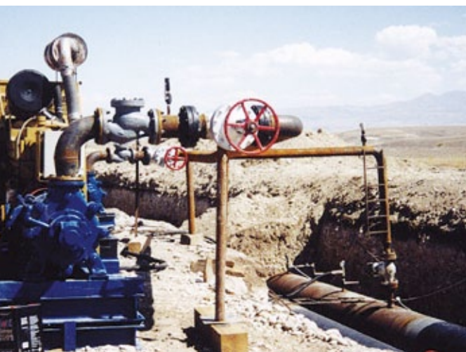
Test pump unit DP3-10 E with gearless drive mounted on industrial chassis
