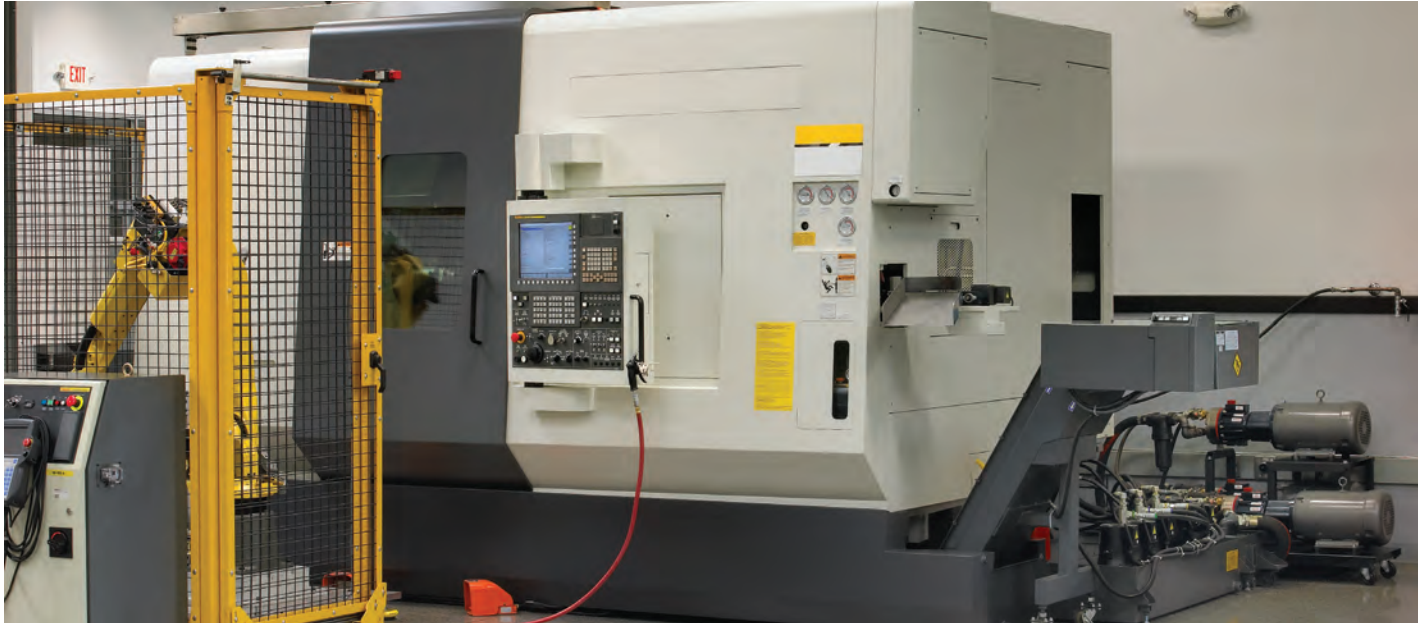
Hydra-Cell pumps deliver high-pressure, controlled flow of machine tool coolant without the need for fine filtration.
