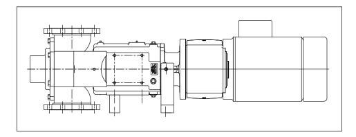
Time-tested Waukesha Cherry-Burrell rotary pump; external circumferential piston (ECP) operating principle.
