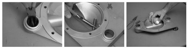
Remove the valve stops [3] and the ball valves [15] out of the side housings [1]. For the AD 32 and AD 50 the use of a screwdriver to remove the valve stops maybe is more convenient.
