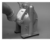
Loosen nuts of the housing bolts on one side of the pump.
