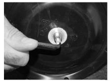
Screw out the set screws, shaft [13a].
