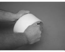
Screw one diaphragm [14] counterclockwise off the shaft [13].
