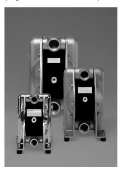
For inflammable liquids as well as for applications in explosionproof areas, Chemicor pumps have to be equipped with a center section in conductive PE instead of the standard Polyamid block. The pump has to be grounded to one of the tapping holes located in the side housings. All other housing parts are connected to the side housing; therefore it is not necessary to ground single parts.
