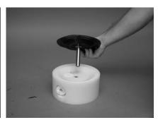
Pull the other diaphragm [14] together with the shaft [13] out of the center block [16].
