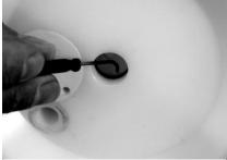
Remove both parts of the shaft piston rings [17] from their grooves carefully (do not damage the edges in the center block; a re-assembly of the same piston rings is impossible; they have to be replaced). Unscrew the muffler [20], the air inlet [18] and the air filter [19] out of the center block [16].
