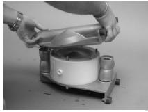
Remove side housing [1] and suction/discharge ports [2].
