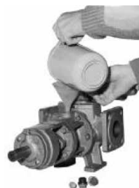
Filling up the pump
