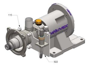
• Remove the pressure switch set and bracket on working table.
