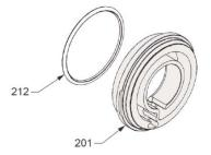
If the 100 nozzle is oriented differently from the standard position (§ 2.1), it is important to orient cylinder 201 as shown here, in other words with the port at the bottom. It is possible to fit the cylinder with the port at the top, but the pump will then not be drainable.
