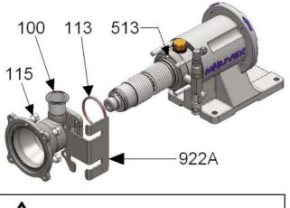
BE CAREFUL NOT TO KNOCK OR SCRATCH THE BELLOWS AND THE PRESSURE SWITCH.
