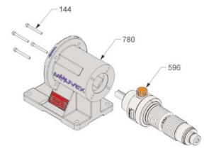
Reassembly is in reverse order. The screws 144 must be fitted using Loctite<sup>®\*</sup> 243 or equivalent thread locking adhesive (tightening torque of the 4 M6 screws : 5,5 Nm).
