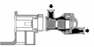
• A centrifuge pump is used for CIP cycles. This centrifugal pump is placed upstream of the SLC pump.
