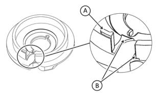
Before putting back the piston on the pump, eliminate these asperities by filing and finishing with fine sandpaper (No 320 grain or equivalent), taking care of not scratching any other surface around. Piston must then look as follows :
