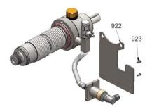
On the spare transmission, remove the 2 screws 921 and the two screws 923 and remove the transport / storage bracket 922B.
