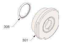
• Insert piston 301 over the transmission hub 596, with the slot of piston 301 opposite the cylinder partition 201.
