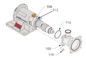
The spare transmissions delivered are equipped with a tubular foam protection. We advise leaving this protection around the bellows until remounting of the piston and cylinder.
