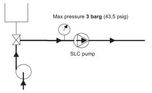
It is preferable not to run the SLC pump during CIP although low speed (< 100 rpm) is acceptable by alternating start/stop operation.
