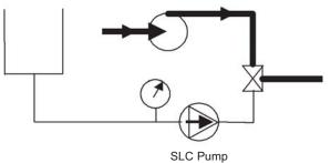
The SLC pump is stopped when cleaning the installation.
