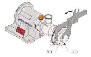
• This operation can be done using MOUVEX tools references 227115 (bracket) and 315361.00 (socket).
