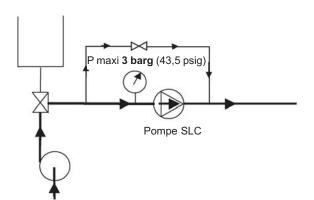
It is preferable not to run the SLC pump during CIP although low speed (< 100 rpm) is acceptable by alternating start/stop operation.
