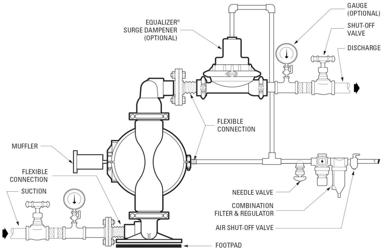
**NOTE:** In the event of a power failure, close the shut-off valve if you do not want the pump to restart when the power returns.
