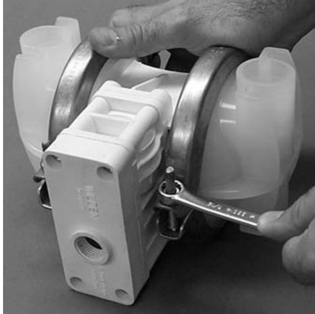
Step 8 Use a 11 mm (7/16") wrench to remove one set of clamp bands that secure one liquid chamber to the one-piece center section.
