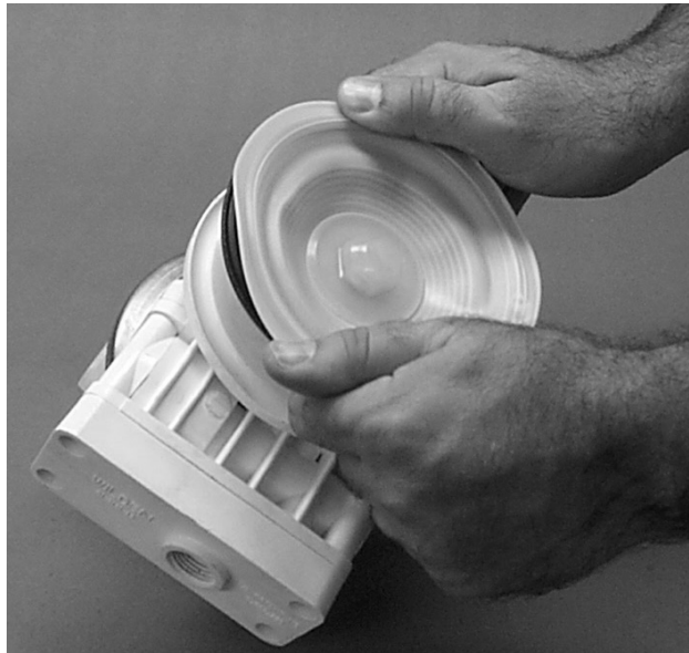
Step 10 Using an adjustable wrench, or by rotating the diaphragm by hand, remove the diaphragm assembly from the center section.
