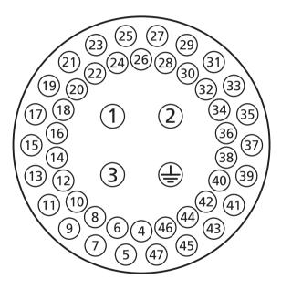
Fig. 7.1.1 Terminal numbers refer to connections as shown on the actuator circuit diagram
