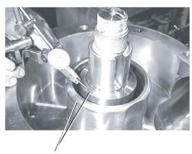
MEASURE BOTH SHAFT S. APPLY SHIM UNDER FRONT BEARING SEAT, IF REQUIRED.
