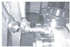
**INSTALL NUTS TO 600 FT.LBS TORQUE**
