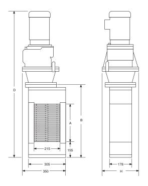
On IP67 & IP68 motor dimension D is increased by 74mm on 1.5kW motors.
