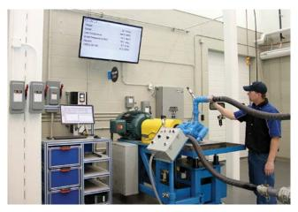
Certified performance testing on a sealless magnetically-coupled pump on one of 8 dynamometers in our newly expanded research lab, allows us to test a full range of pump capabilities on liquids at the customer's viscosity.
