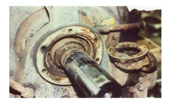
Most bearing failures are not caused by a bearing manufacturing defect. Bearing failure mode is usually caused by lubricant breakdown or above-normal bearing loads.
